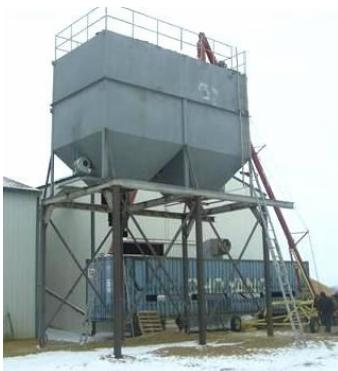
*In 2005, Prairie Bioenergy became the first Canadian producer of densified crop residues for energy. Their biomass cubes are loaded into an overhead bin for bulk loading into trucks.*
