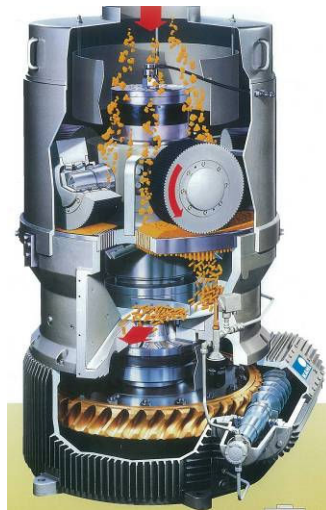
Figure 3: Kahl Corporation flat die pelleting process
