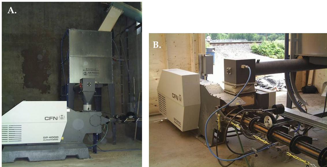
Figure 8. Briquetting System; (A) West Fraser Westpine MDF sheet plant; (B) Federated plywood plant (Photo courtesy of Wayne Winkler).
