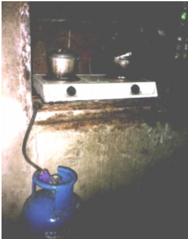
Photo 2.7. A typical LPG cooking stove with bottled gas, a system used in more than 4 million households in the Philippines.
