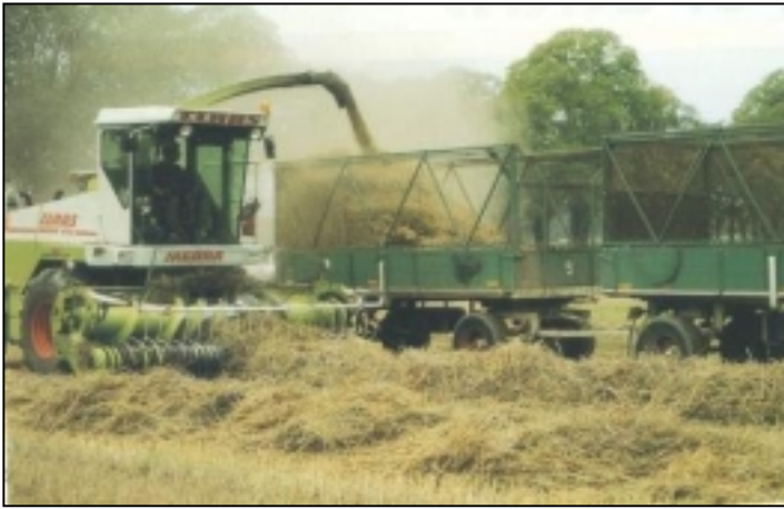
Photo 3.6: A self-propelled chaff cutter can blow straw into wagons or open transport trucks that can take the materials directly to the processing plant (Centre for Biomass Technology, 1998).
