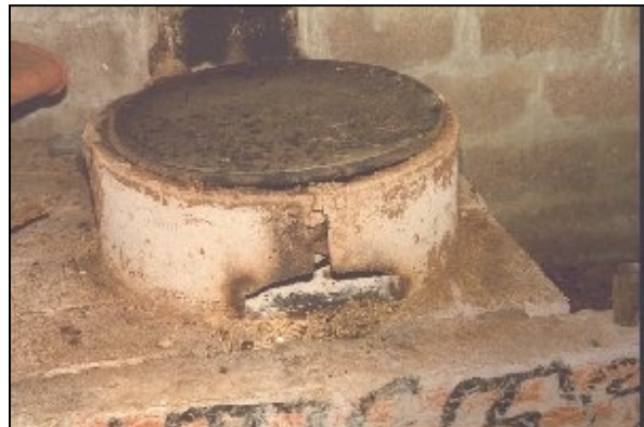
Photo 1. The Mirte stove efficiently bakes household bread in Ethiopia (ESB, online information).
