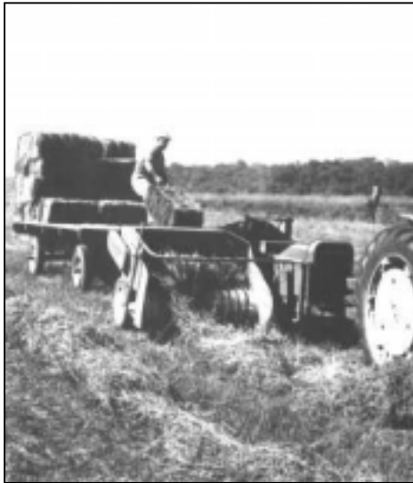
Photo 3.2. Small square baler with flatbed trailer in tow (hay bales)
