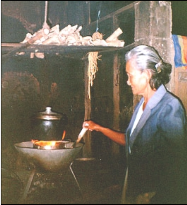
Photo 2.10. High efficiency stoves completely burn the fuel being used and effectively transfer the heat to the pot, thus reducing the amount of fuel needed for cooking. An important fuel saving feature is an adjustable heat output, for boiling then simmering rice. Sufficient energy is needed to replace heat losses during the latter part of the cooking cycle. Greater control of heat output would improve user acceptance of improved biomass cooking stoves.
