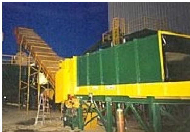
Photo 3.10. An industrial bale breaker from Newhouse Manufacturing in Oregon produces an output of 10 tonnes/hour for large square bales, has an 80 horsepower motor, and produces a chop of 1.5 to 6 inches in length. The cost of the device is approximately $50,000 US.
