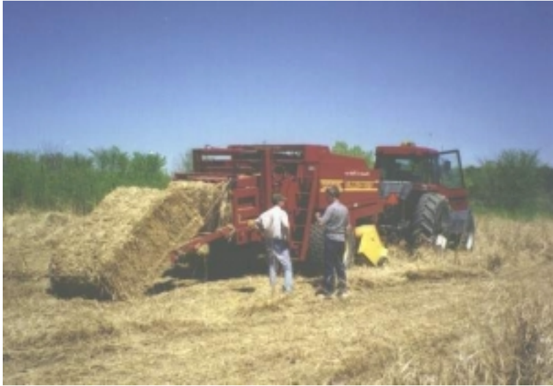
Photo 3.5. A big square baler produces rectangular bales 3' x 4' x 8' in dimension which have a density of 150-175 kg/m 3 .
