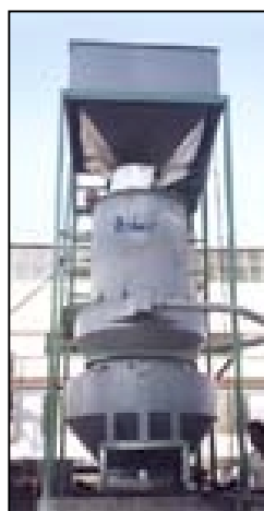
Photos 2.1 and 2.2: This 100 kW electric system in India is powered by rice hulls.
