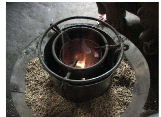
Figure 3. The Mayon Turbo Stove offers the clean combustion of a low cost, locally available resource.
