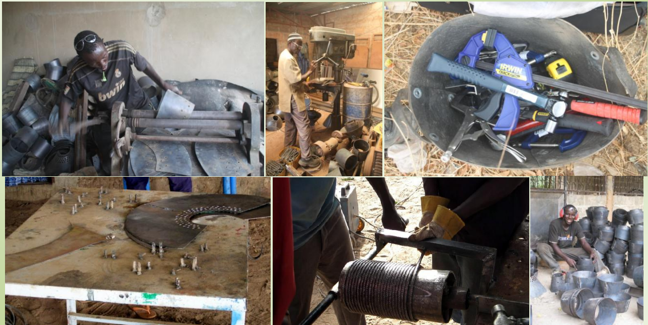
Clockwise from top left: Rolling hoppers in Kaolack, Drill press in Sukuta, Hand tools in Wack Ngouna, MTS Jig in Wack Ngouna Rebar rolling in Farafeni, Fitting cones together Njawara.
