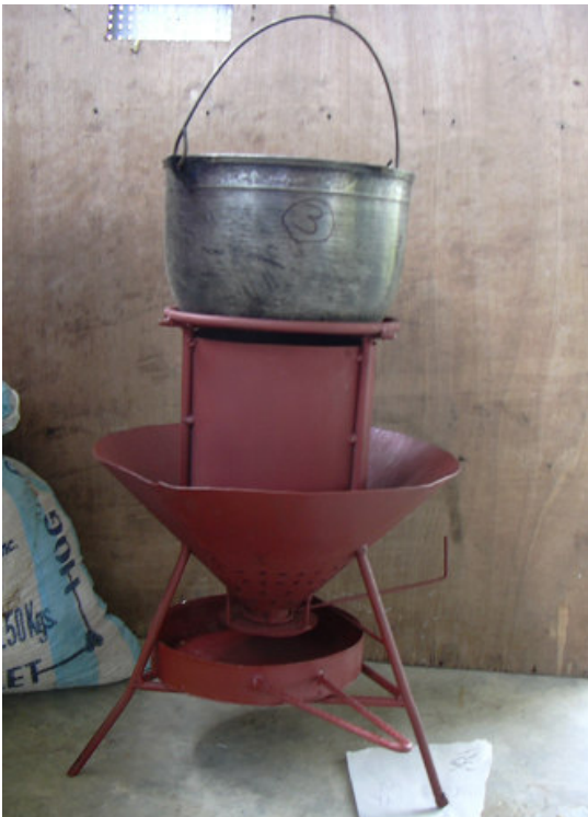
Figure 4: CPU Conical Grate Rice Hull Stove (stove model #3)
