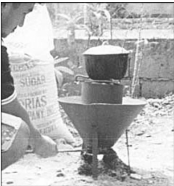
A good flame can be maintained by tapping on the stove to release ash and allow fresh rice hulls to fall into the fuel bed.
