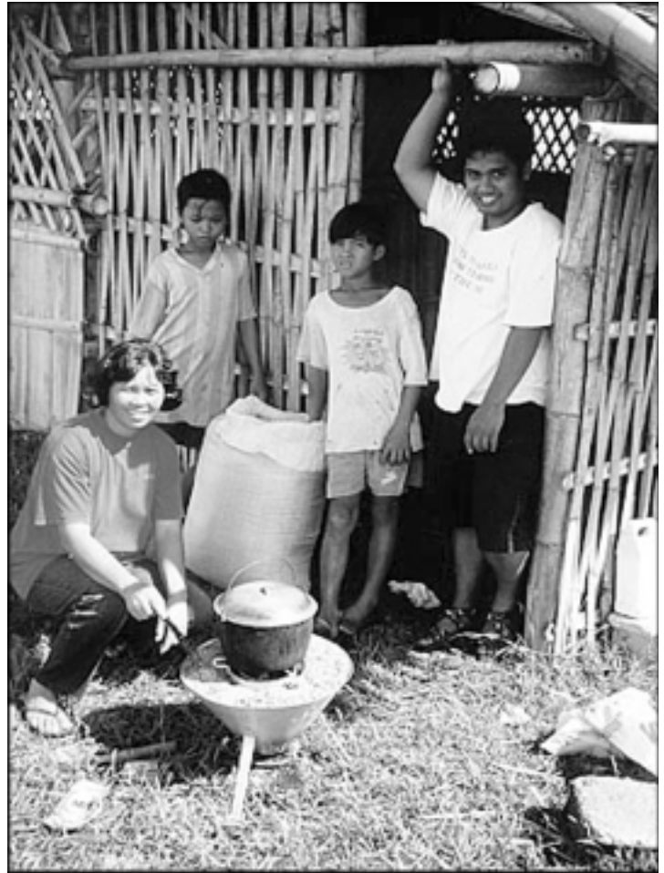
A woman in Negros cooks her lunch on the rice hull cooker, collecting the ash on the ground.
