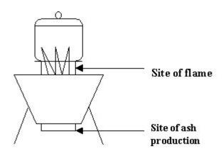
5. If the stove goes out while cooking it is almost always because of lack of fuel. If tapping to introduce new fuel does not immediately restart the fire, the opening between the outer fuel bin and centrepiece can be reopened. Usually the glowing embers will restart the cooker if an air draft and fresh fuel are present. The stove can also be restarted as indicated in steps 1-3 above.
